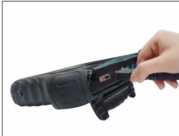
Fig. X-1 Connecting to DLC Connector
