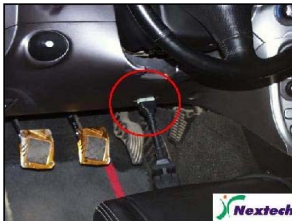
Fig. X-2 Connecting to Vehicle Side Connector
