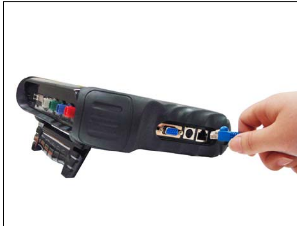
Fig. XIII-1 LAN Cable Connecting Method
