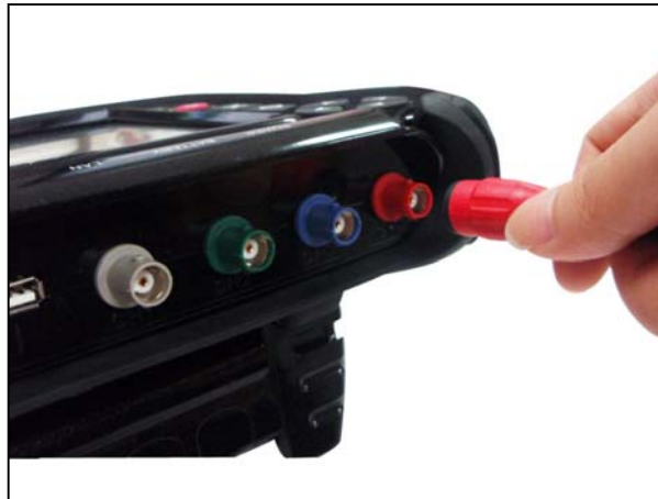
Fig. XIV-1 Scope Cable Connecting Method 1
