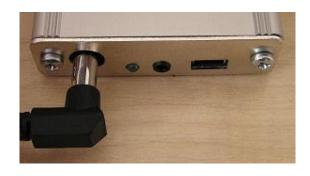
USB power from PC - 5V, 100mA. Always must be connected because USB cable is used for Device – PC communication. Is enough for small power consumption operations (i.e. EEPROM read/write)
