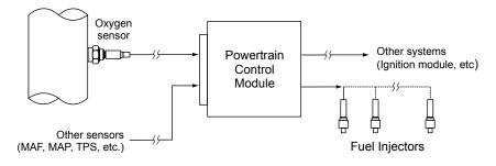
Fig. 4 - Oxygen sensor function
