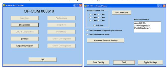
Since Opel uses many pin in the OBD connector, the diagnostic interface works as a multiplexer, and selects the appropriate pin for communication.
