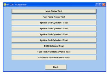
You will get a feedback on the state of the activated output. This will helps you to find the failed components more easily.
